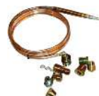
THERMOCOUPLE SUPER UNIVERSAL T140/900AT Aluminised tip 900mm
